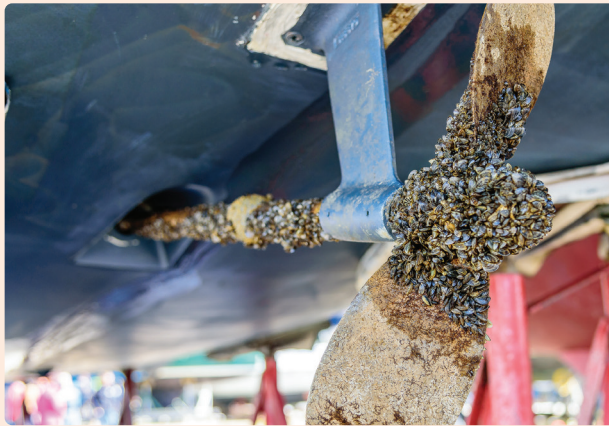
Zebra mussel fouling in pipes and on vessel
