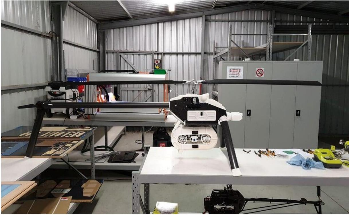
*Autonomous Technology Drone Fitted with Bait Delivery System*
