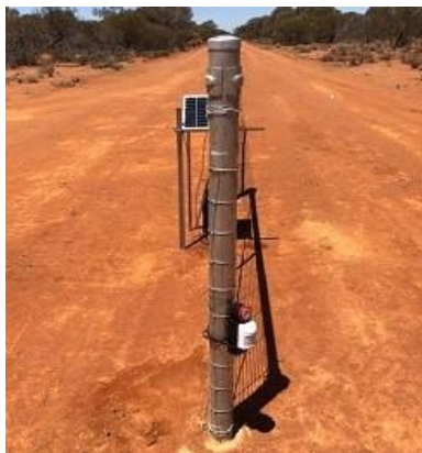
Squawker and howler box set-ups including deep cycle battery, solar panel and squawker devices deployed separately. They are easily moved.
