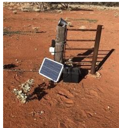
Squawker and howler box set-ups including deep cycle battery, solar panel and squawker devices deployed separately. They are easily moved.
