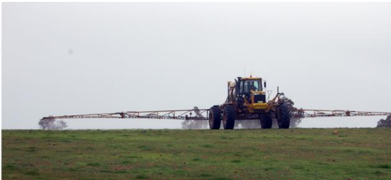
A self-propelled sprayer. Photo courtesy of DPIRD.
